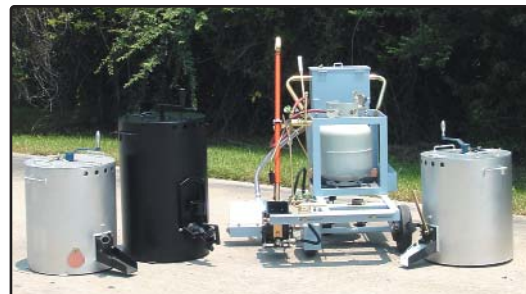
Tank is removed in approximately 45 seconds and may be replaced with another color tank or bitumen tank.
