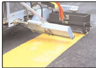
All steel extrusion dies up to 18" wide.
